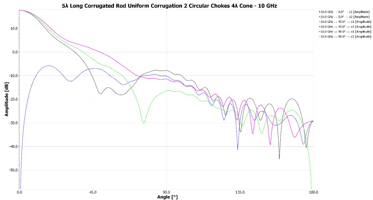
Figure 10-4.1.17 Center Frequency 5\lambda Long Uniform Amplitude Corrugated Rod inside a 4\lambda Long 20^\circ flare Cone
