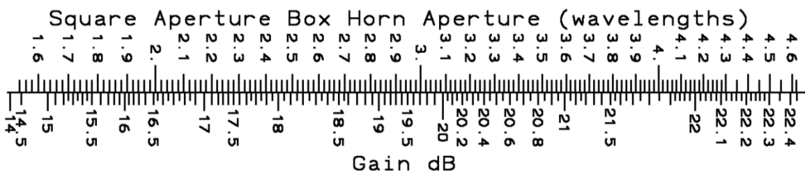
Scale 7-7.1.1 Box Horn Aperture given Gain
