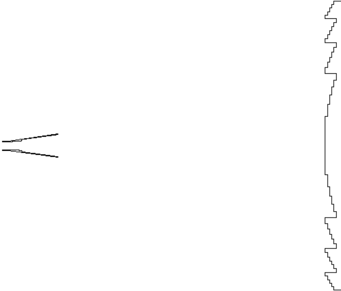
Figure 9-2.2.1 Dielectric Zoned Plate Lens with P = 6 ( \lambda/P or \lambda/6 ) steps fed by Potter Horn
