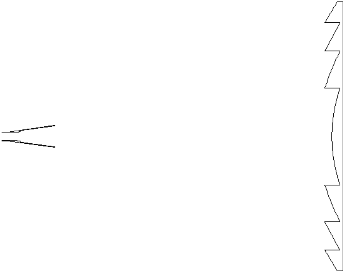
Figure 9-2.2.2 Flat Radiation Side Dielectric Zoned Lens with continuous surfaces fed by Potter Horn
