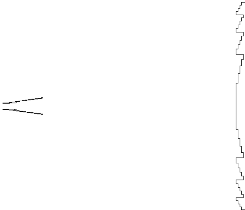
Figure 9-2.2.4 f/D = 0.937 Dielectric Zoned Plate Lens with P = 5 ( \lambda/P or \lambda/5 ) steps fed by 16 dB Potter Horn
