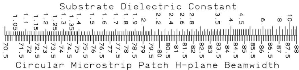
Scale 6-8 H-plane Beamwidth of Circular Patch on infinite ground plane
