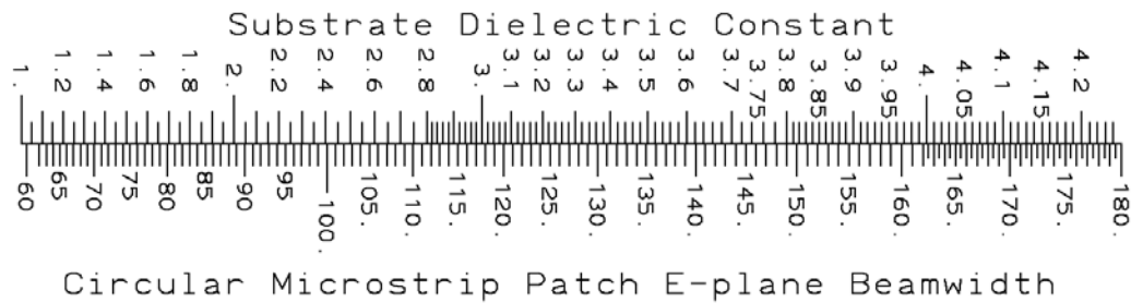
Scale 6-7 E-plane Beamwidth of Circular Patch on infinite ground plane
