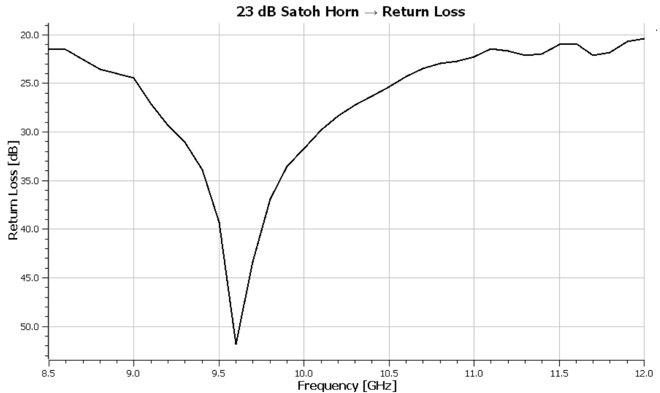
23 dB Gain Satoh Horn Return Loss versus Frequency
